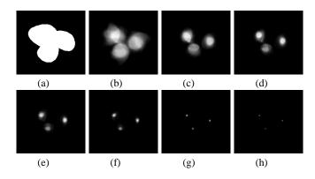
**Fig. 2.** Detection of radial symmetries for a synthetic image with multiple overlapping objects: (a) original image; (b)-(g) voting landscape at each iteration; and (h) final localization of centers of mass.
